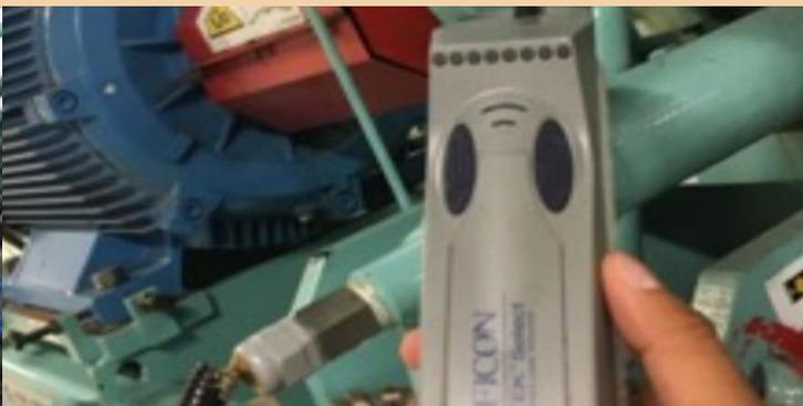
In our inspections we check circuits and components that show any risk of leaking using proper detection devices.
